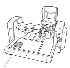
Place the plate on the adhesive sheet, then press down on it from above to anchor it securely.
